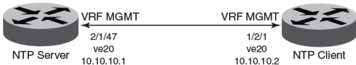
FIGURE 3 Use case 1: Management VRF forwarding with one client and one server on ve
